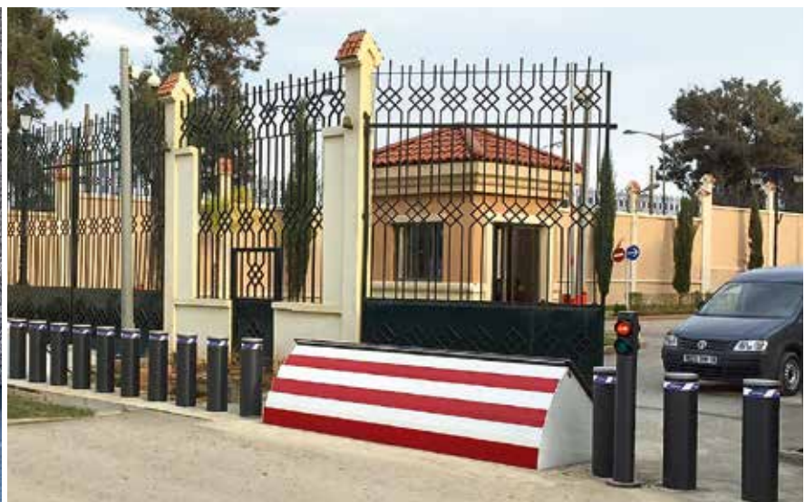
No access: This entrance is protected with fixed bollards and a road blocker.
